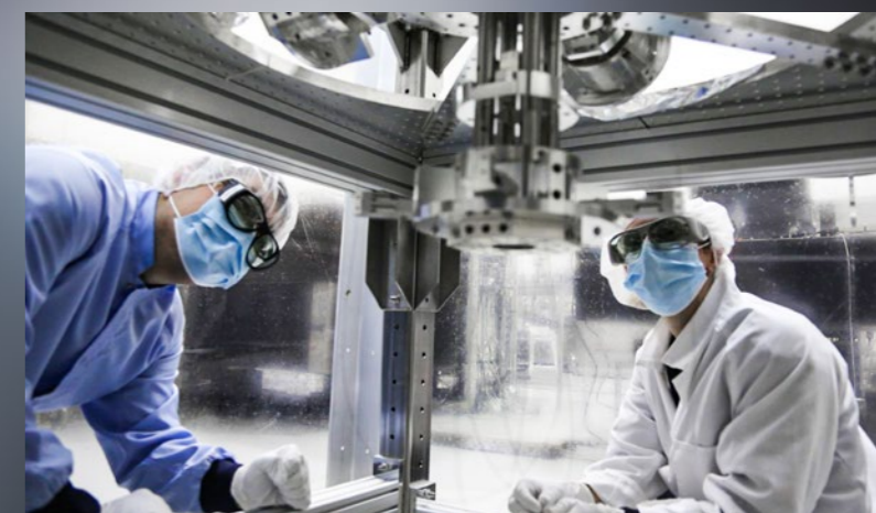
Research Assistant Lauren Sarre and Dr Sheon Chua inspecting the recently assembled Penultimate Mass. Delicate balancing and precise mass locations are required to make the suspension work properly. Image credit: Bram Slagmolen, OzGrav ANU
