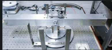
Fully assembled tilt sensor. Credit: Joshua McCann, OzGrav UWA
