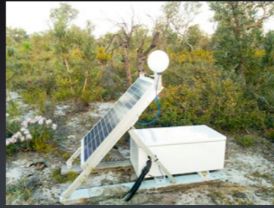
A standalone seismic station deployed in Gingin Gravity Precinct with the data acquisition box and wireless transmitter. The seismometer is buried underground.
