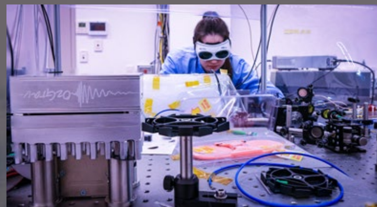
Georgia Bolingbroke, PhD student at University of Adelaide, is assembling and testing the distributed Bragg reflector laser. Credit: Huy Tuong Cao, OzGrav Adelaide
