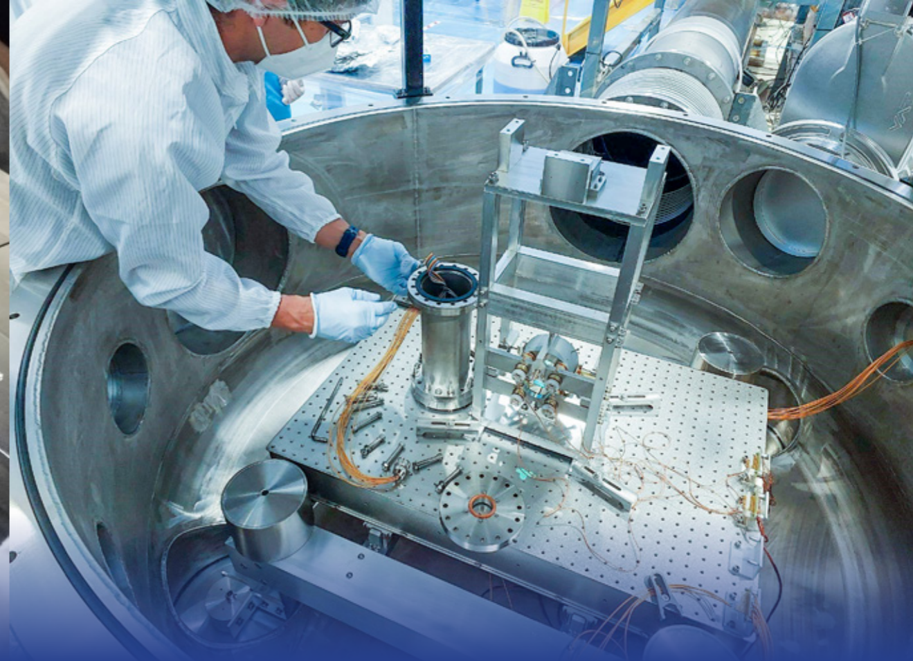
Carl Blair installing the seismometers for the piezo pre-isolated table for use on 7m 2 μm suspended cavity (pictured) and 80m coupled cavity experiments. Credit Jian Liu, OzGrav-UWA.
