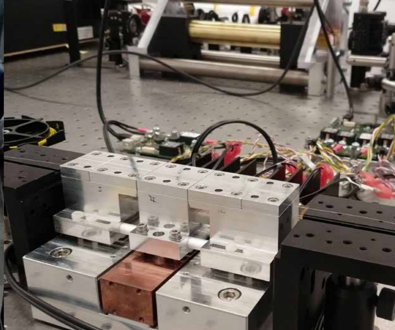
Image: A prototype of the 2µm fiber laser being developed for third-generation detectors with cryogenic silicon mirrors. Credit: Sebastian Ng, OzGrav University of Adelaide.
