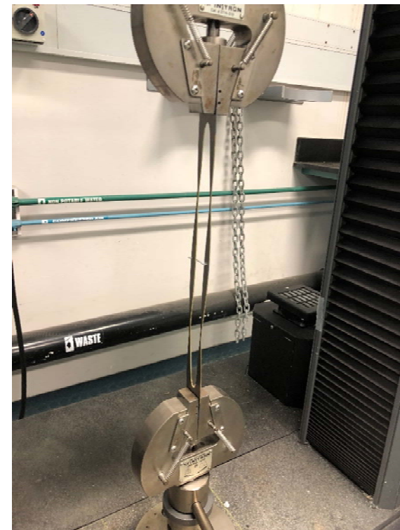
Contoured Euler springs in compression tester
